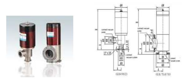
This electro-magnetic vacuum gas valve is a special valve installed in rotary vane vacuum pump. The valve and pump should be connected in the same power. The pump start / stop directly controls the valve open / close. When the pump stops working or there is a sudden interruption of the power supply, the valve will automatically close the vacuum system and fills gas into pump through the pump gas inlet. In this way, it prevents the pump oil return to the vacuum system.
