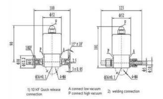
This electro-magnetic high-vacuum gas valve connects with high & low vacuum system. When the valve is electrified, it connects together P & A end pipeline. When the valve outraged, the valve plate close and turn off the P &A end pipeline in order to protect the vacuum degree, At the same time fills gas to A end through F end.
