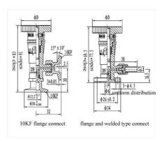
This T series high vacuum micro metering valve(also known as vacuum needle valve)adjust taper needle and length of gap by screw drive, change conductance number of valve seat, is used to fill gas into the vacuum system and could adjust air suction flow exactly, in order to control and regulating vacuum degree in system. Applicable medium can be air without particles of dust and noncorrosive gases.
