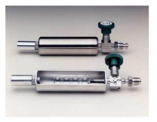
The CLP Helium Calibrated Leaks are high-precision Standards for use in critical calibrations of leak detectors and systems, in Ultra-High Vacuum systems, and as Transfer Standards for calibrating other Helium Leaks. They feature all-welded stainless steel construction, a premium all-metal shut-off valve, a glass-permeation leak element, and are bakeable for UHV applications.
