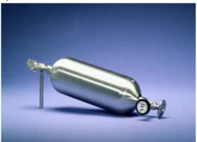
The GPC Model Helium Calibrated Leak Standards have crimped stainless-steel capillary leak elements and are widely used to tune and calibrate helium mass-spectrometer leak detectors and leak testing systems. They are part of a family of Helium Calibrators offered by Unique Vacuum Solutions including the GPP, GPPT and CLP Models detailed in other brochures. Together they cover a wide range of leak rates from 10<sup>-12</sup> to 10<sup>-2</sup> atm-cc/sec and larger.
