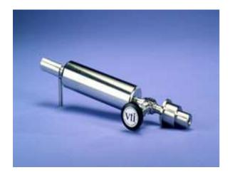
These GPPT Model Helium Calibrated Leak Standards have Teflon®-permeation type leak elements and are widely used to tune and calibrate helium mass spectrometer leak detectors and leak testing systems. They are part of a family of Calibrators including the GPP, GPC and CLP Models offered by Unique Vacuum Solutions that cover leak rates from 10<sup>-12</sup> up to 10<sup>-3</sup> atm-cc/sec and larger.
