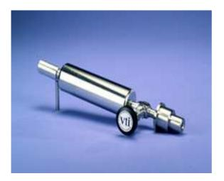
These GPP Model Helium Calibrated Leak Standards have glass-permeation type leak elements and are the most common ones used to tune and calibrate helium mass spectrometer leak detectors, leak testing systems and vacuum systems. They are part of a family of Calibrators including the GPPT, GPC and CLP Models that cover leak rates from 10<sup>-12</sup> up to 10<sup>-3</sup> atm-cc/sec and larger.
