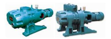
It is a mechanical pump with high evacuating speed also referred to as mechanical booster pump. The rotors rotate synchronously in opposite directions and high speeding. The pump cannot be used singly, it must be used as boosters combined with a backing pump such as a rotary piston or a rotary vane vacuum pump, or a liquid ring vacuum pump. These vacuum systems can get higher vacuum, a stable, fairly high pumping speed can be gained in effective pressure range.
